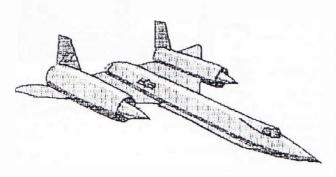
Powered by Pratt & Whitney turbojets, the first aircraft flew in 1962, almost three years after the initial proposal. It was 102 feet long, had a 57 foot span, could tly at Mach 3.2 and reach an altitude of around 85,000 feet with a range of 4,100 miles. Designed as a long-range interceptor
