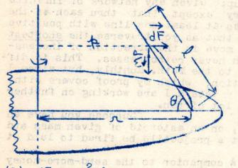
As will be recalled, the disc spins about the vertical axis with angular velocity w. A rod of length & and mass distribution P(x) is hinged to the disc at distance r from the axis. To find the angle,  $\theta$ , at which the centrifugal force can hold the rod u p off the disc against gravity.
