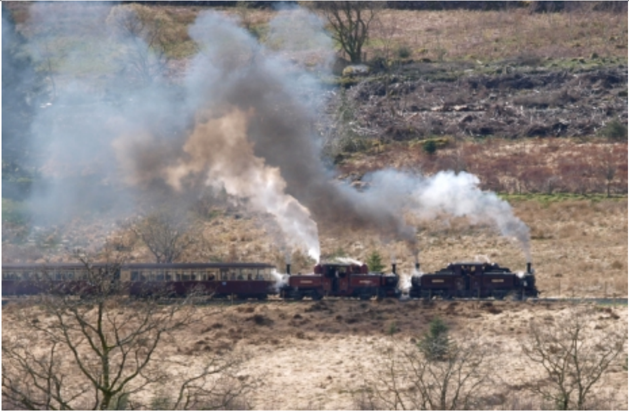
The Festiniog Railway in North Wales helped develop a special type of articulated locomotive, the Fairlie — named for its inventor — to double the power available to haul slate wagons whilst only needing one crew. This was a special train over the newly reopened Welsh Highland Railway in 2011.
