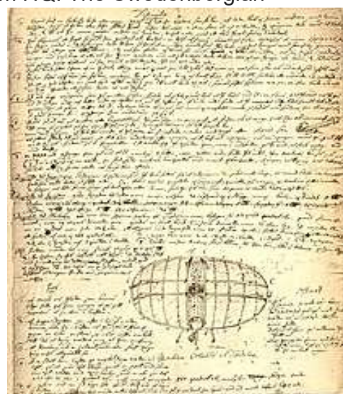
Swedenborg notes, with a drawing of his "flying machine". The elliptical wing was aero-dynamically on the right track and he understood that centre of gravity must be low. But it would take a couple of centuries of tests and finding a light enough power source for real flying.
