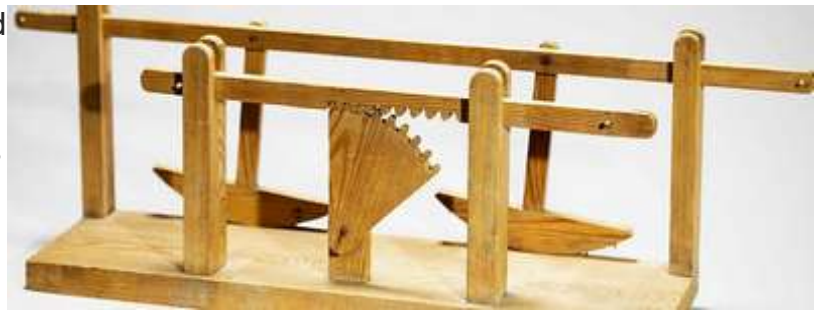
An entry of Polhem's mechanical alphabet, dealing with how every type of motion can be transformed to another type.
