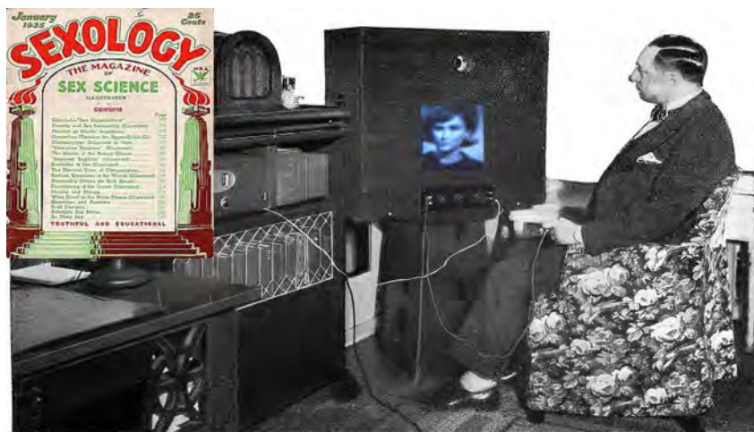
H. Gernsback, Editor of RADIO NEWS, receiving the television broadcasts from WRNY at his home in New York City, with the simple apparatus described in this article. For purposes of the test, the neon tube and loud speaker were connected in series temporarily, with successful operation simultaneously.
